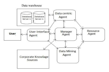
Figure 2.Block diagram of agents based distributed data mining system
