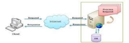
Fig.5. Three tier architecture of distributed data mining
