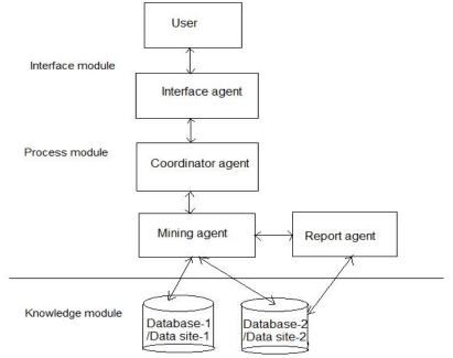
Fig. 4. Architecture of agent based distributed data mining
